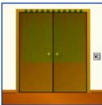
Overhead Sensor Array The overhead sensor array detects side-by-side passages through the doorway.
